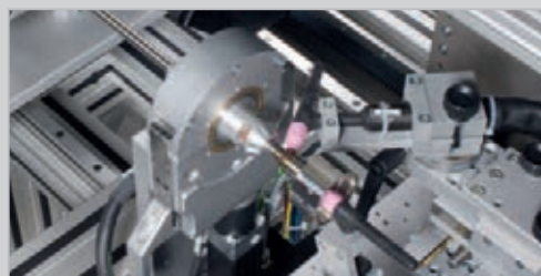
Simultaneous TIG circular seam welding
